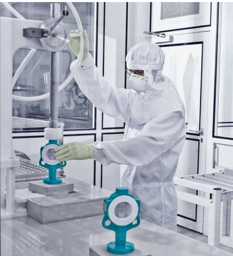
Assembly of the Bianca butterfly valve in the clean room
