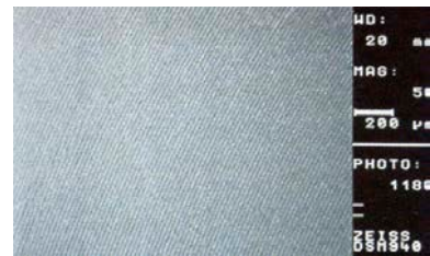
50x enlargement of the surface of a machined ULTRAFLO ® liner
