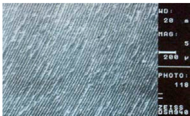
50x enlargement of the surface of a machined PTFE liner
