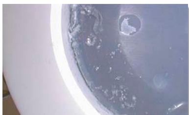
Abrasion of a standard PTFE liner
