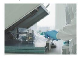
The clean room is cleaned regularly, the air flow is strictly controlled and workers wear special work clothes and latex gloves throughout the production process.
