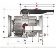
**VKDOAC**DUAL BLOCK® 2-way ball valve with fixed flanges, drilled ANSI B16.5 cl.150 #FF. Face to face according to EN 558-1
