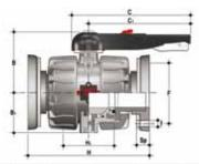
DUAL BLOCK® 2-way ball valve with fixed flanges, drilled EN/ISO/DIN PN10/16. Face to face according to EN 558-1
