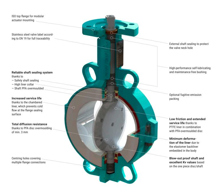
The high liner collar, the PFA disc overmoulding on the shaft as well as a lifetime preloaded safety shaft sealing guarantee both excellent primary and long-lasting secondary shaft sealing, even for greater operating cycles and at high temperatures.
