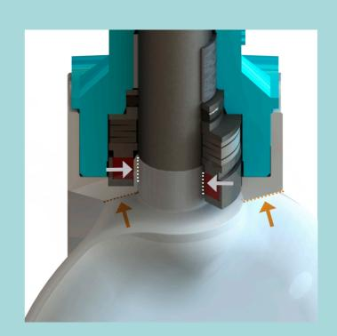
•••••• Primary sealing Secondary sealing
