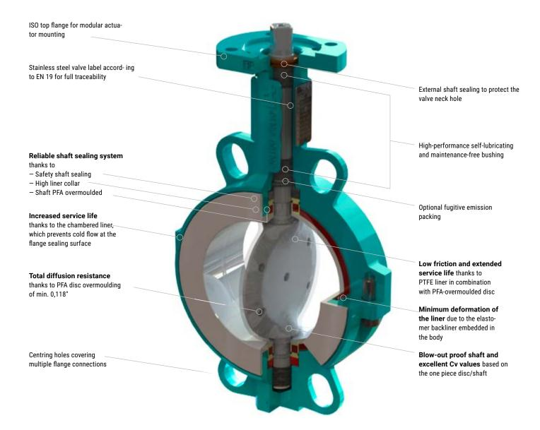
The high liner collar, the PFA disc overmoulding on the shaft as well as a life-time preloaded safety shaft sealing guarantee both excellent primary and long-lasting secondary shaft sealing, even for greater operating cycles and at high temperatures.
