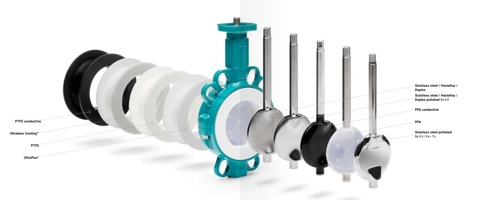
Ranging from mirror-polished stainless steel discs with high-purity Ultraflon® liners for pharmaceutical applications to PFA-coated discs with PTFE liners for the highly corrosive chemical industry - the Bianca butterfly valve can be individually configured for a wide range of applications. High quality and safe and reliable operation are always paramount. Bianca
