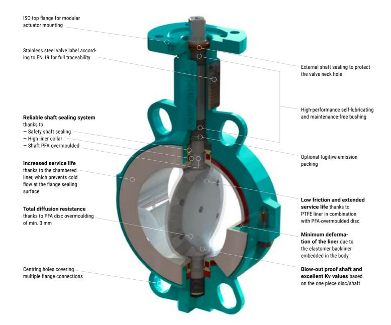
The high liner collar, the PFA disc overmoulding on the shaft as well as a life-time preloaded safety shaft sealing guarantee both excellent primary and long-lasting secondary shaft sealing, even for greater operating cycles and at high temperatures.
