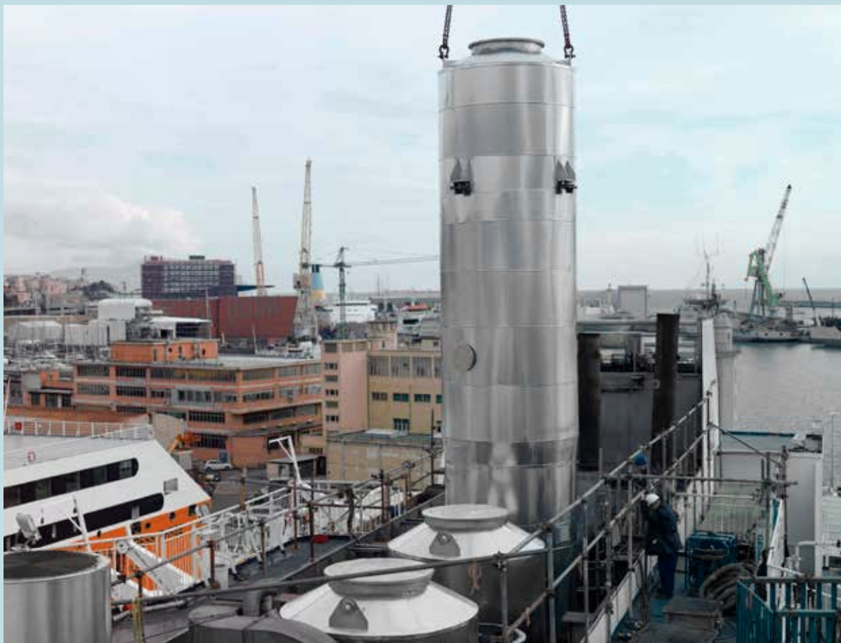
Marine DeSOx system (Image: Courtesy of Ecospray Technologies)
